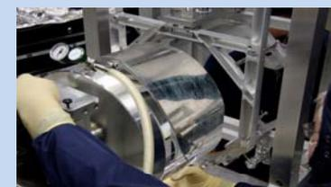
Right: Inserting the silica test mass, January 2009, into the quad structure with the ergo arm.
