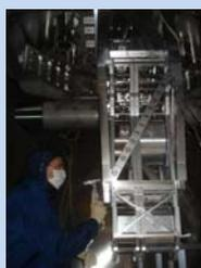
Upper picture: Modal analysis of the quad structure on the ISI. A force sensing hammer is used to measure transfer functions between various points on the structure and the accelerometer location. Information about not only the frequency, but shape of each mode of vibration can be extracted from these measurements. The goal is to identify the modes that limit the ISI's seismic isolation performance.
