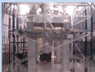
The ISI and quad together on the test stand at LASTI where they were assembled before they went into the BSC.
