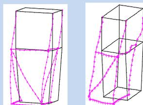
Upper Left: Measurement of the lowest frequency (81 Hz) flagpole mode of the quad structure measured using the modal testing technique. This picture shows the shape of the deformation of this mode.
