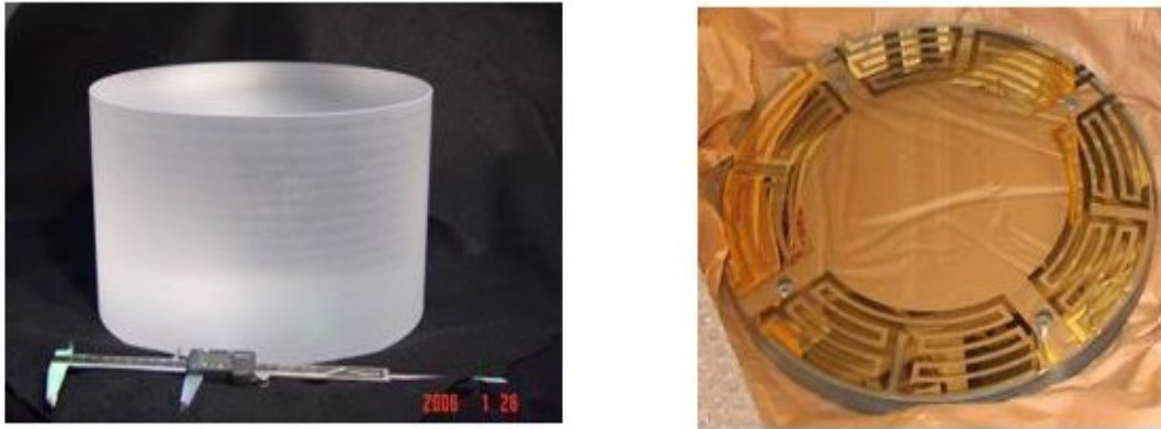
Figure 9 Left: full-size silica test mass (unpolished) procured with UK funding. Right: gold coated glass plate for testing electrostatic actuation in the controls prototype quadruple suspension
