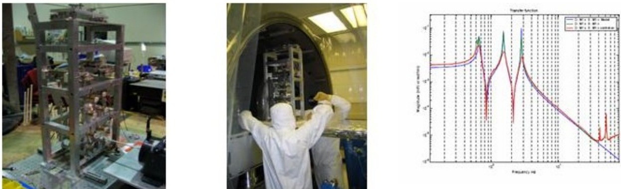
Figure 10 Left and middle: prototype modecleaner mirror triple suspension being bench tested and being installed for further test at the LASTI facility. Right: Longitudinal transfer function top mass drive to top mass position for modecleaner -green (damping off, red (damping on), blue: MATLAB model
