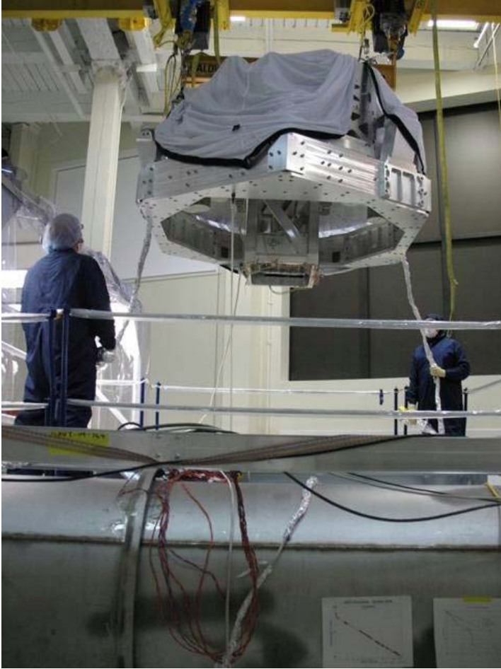
Figure 7: BSC Seismic Isolation prototype , being installed in the test mass vacuum chamber at the MIT LASTI testbed. The upper section of the suspension can be seen at the bottom center of the isolator.
