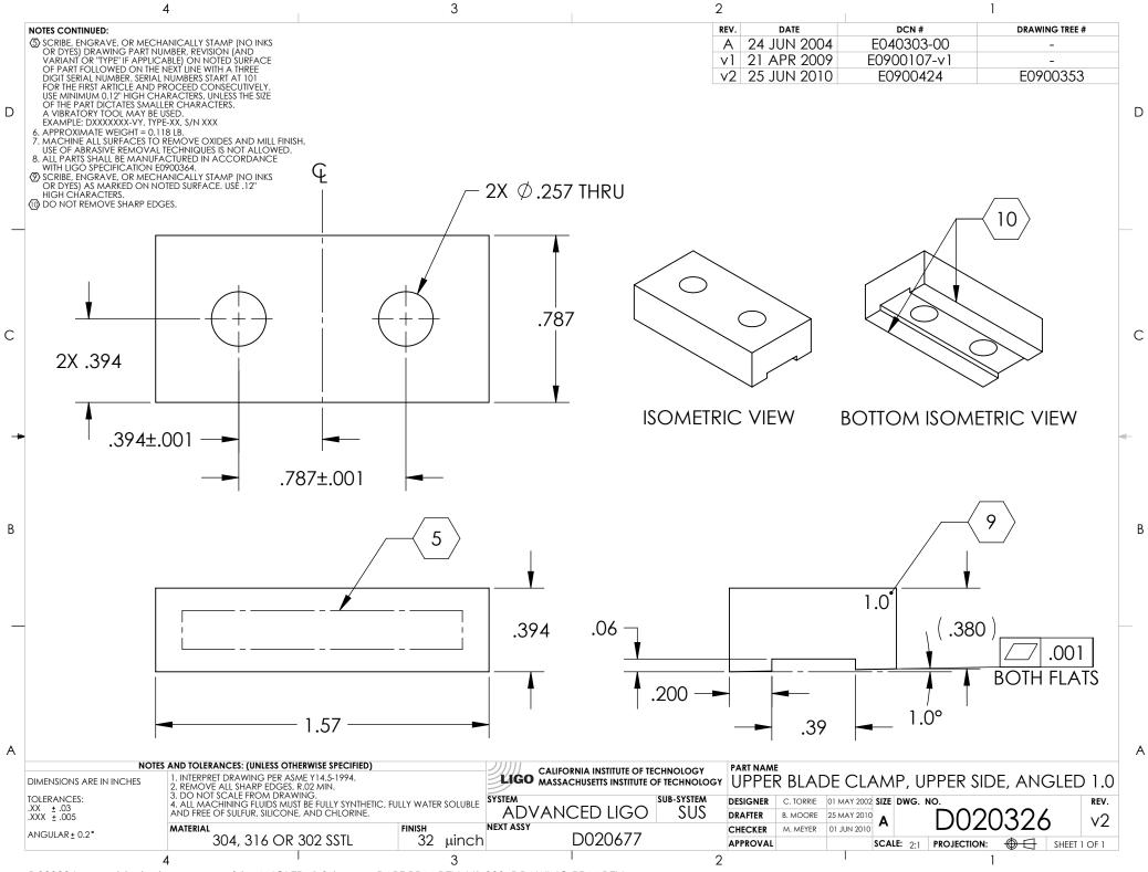
D020326\_upperbladeclamp\_upperside\_ANGLED\_1.0degree, PART PDM REV: V1-000, DRAWING PDM REV:
