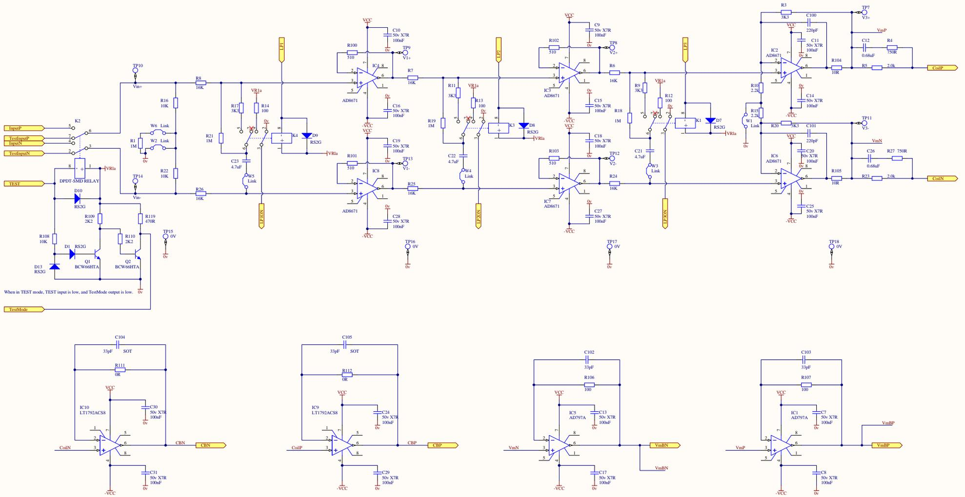
When in TEST mode, TEST input is low, and TestMode output is low.
