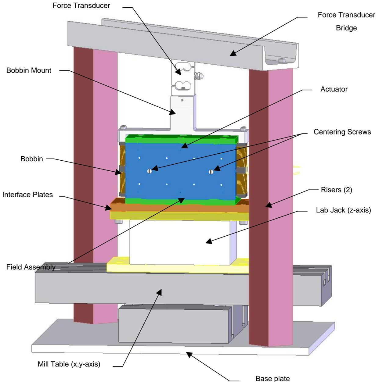
Aluminum channel (Force Transducer Bridge) is mounted on top of two square tube Risers which are in turn anchored to a base plate. The bobbin is attached to a force transducer through a bobbin mount and subsequently to the Aluminum channel. This arrangement fixes the bobbin at a known position (nominally 0,0,0). The mill table-lab jack combination positions the field assembly in the x, y and z axes respectively.
