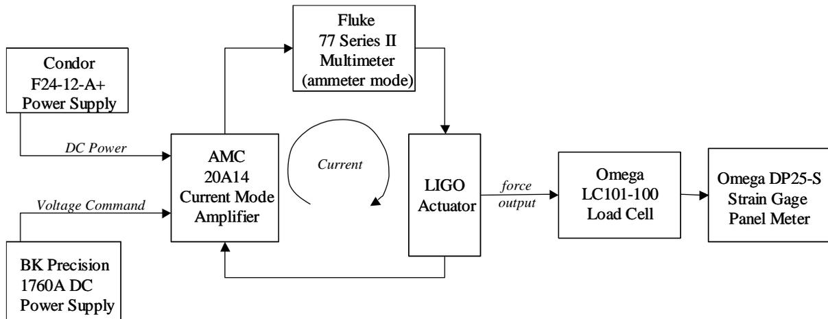
The process for the test procedure is as follows. Before testing, the resistance of the coil is measured to verify proper conductivity. The ambient air temperature is also recorded. With the actuator centered in its housing, the current supplied to the actuator is increased until the maximum specified force output is measured by the load cell.
