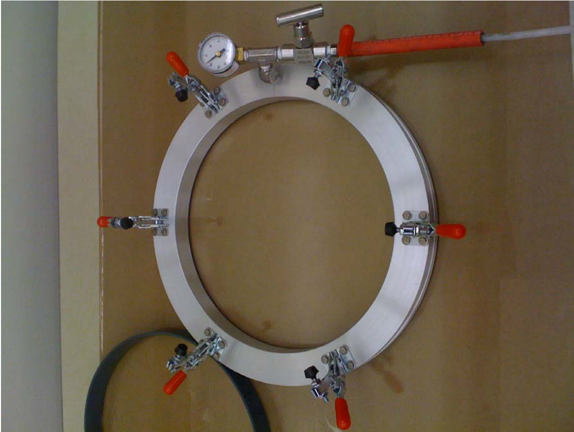
Vacuum Frisbee with the inner o-ring not inserted. Vacuum is 17 inHg, holding for a day+ with the valve closed, pump off, but does not hold for the weekend. The substrate is just a clean piece of plateglass.
