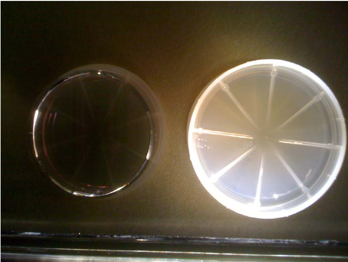
Both cleaned with nc-FC brushed + N2 Ionizer. One immediately covered, other left exposed. Time = 0.
