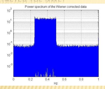
Full band (1 Hz), selected part and histogram of the Wiener filtered data power spectrum.
