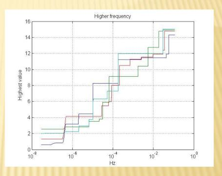
The graph shows the maximum of the normalized absolute square of the 4 basic matched filters applied at frequencies near the apparent frequency. The abscissa is the distance from the apparent frequency.
