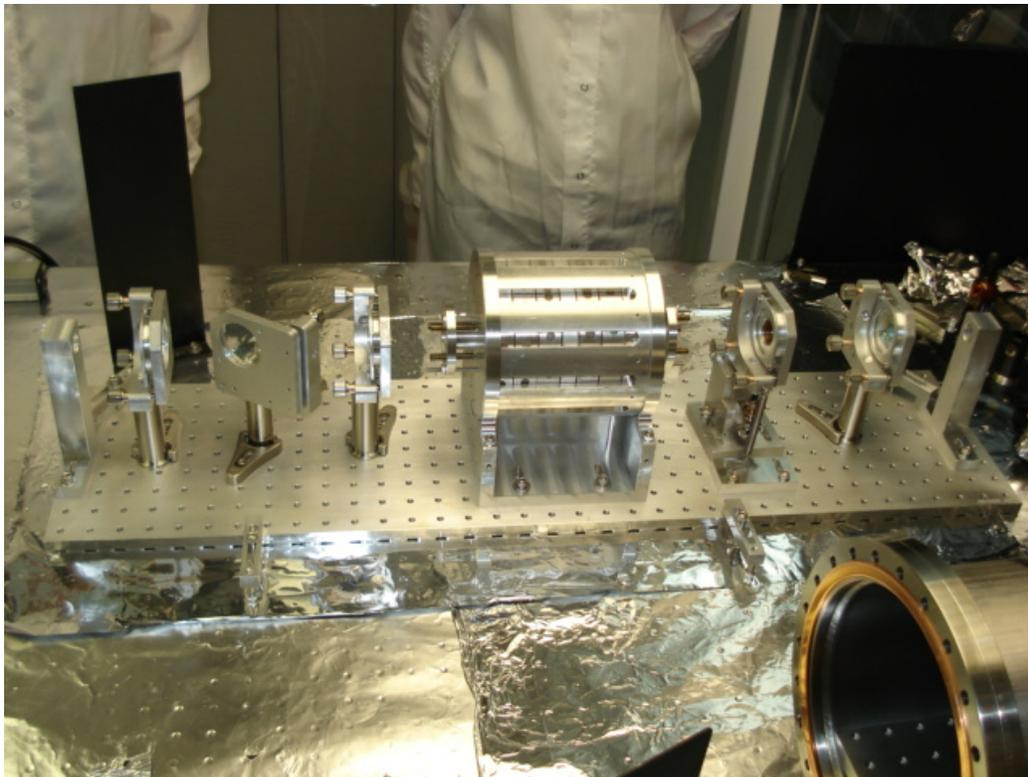
Turn off the IPG laser and store the Faraday assembly until ready for installation in the vacuum.
