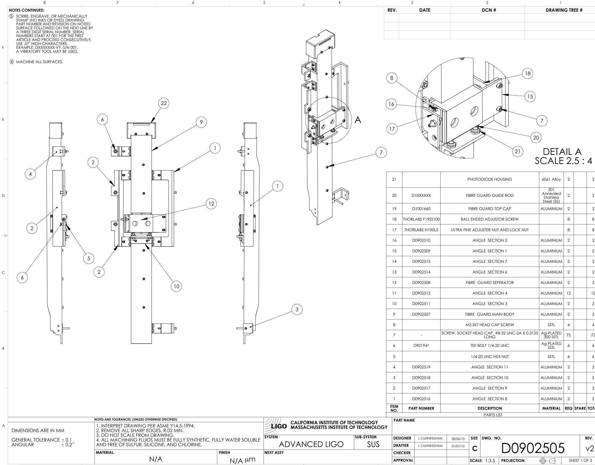
8 D0902505-v2 Fibre Guard Assembly all parts, PART PDM REV: V1, DRAWING PDM REV:
