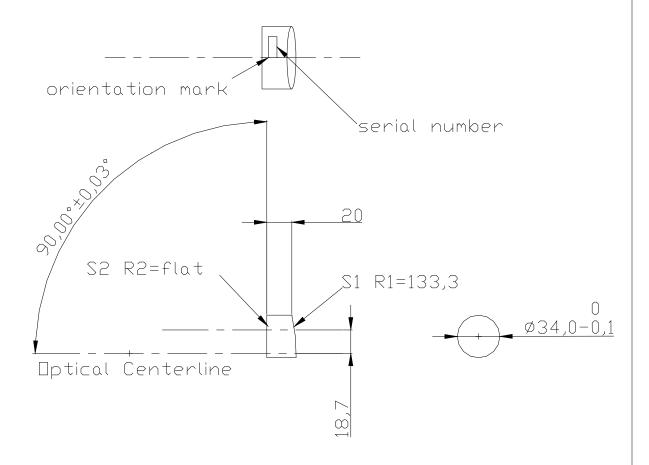
Figure 1: Mirror drawing, parabolic secondary mirror
