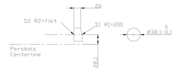
Figure 1: Mirror drawing, parabolic secondary mirror
