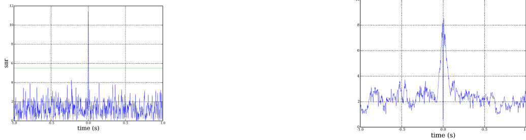
Figure 6. Signal-To-Noise Ratio (left) and \chi^2 (right) time series obtained after match-filtering the Livingston data containing the Candidate G (simulated inspiral gravitational-wave signal). The time origin on the x axis coincides with the time of the inspiral trigger.
