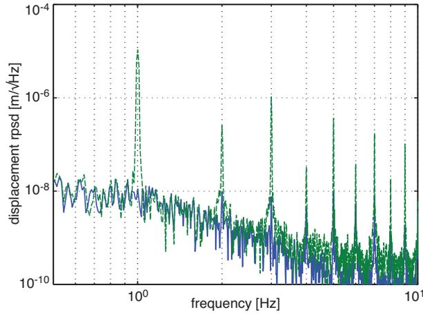
Fig. 6. Root power spectral density of data from Figure 5. The ratio of the 1 Hz scan signal sets an upper bound on the crosstalk between channels at less than  $10^{-3}$  ( $\alpha > 1000$ ).
