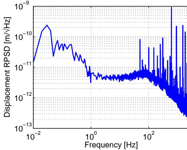
Fig. 3. Spectral density of the DI measurement of cavity displacement when the cavity is locked using PDH locking. Spectral density averaged for clarity (3x for  $0.1 > f > 1$  Hz, and 10x for  $f > 1$  Hz)
