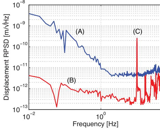
Fig. 4. Comparison of DI readout (A) and digital implementation of PDH readout (B) with the cavity locked using the analog PDH system. The feature (C) is a calibration peak used to scale the digital PDH readout. The lower noise level of (B) indicates good agreement of analog and digital PDH systems and rules out analog electronic noise in the mixer and controller as the limitation of the DI measurement.
