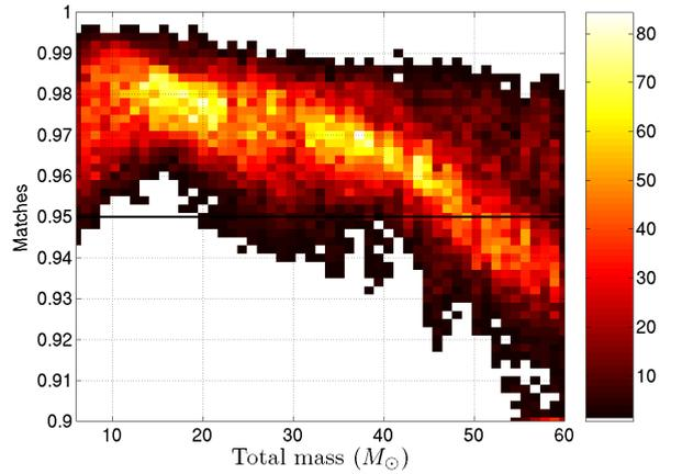
FIG. 6: Distribution of the efficiency versus the total mass. The simulation consisted in  $N_s = 40,000$  injections. The lower cut-off frequency of the injections and the BCV templates is 50 Hz, as in S4 BBH search. For convenience (same scale as in figure 5), we do not show simulated injections with total mass above  $60 M_\odot$  and matches below 90% (see text for details).
