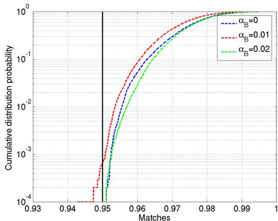
FIG. 2: Template bank efficiencies versus  $\alpha_B$  parameter. The  $\alpha_B$  parameter does not significantly affect the matches. Most of them are above the minimal match of 95%, and more importantly the three distributions are close to each other. In this example, we used the same simulation parameters as in section IV A, and EOB injections.
