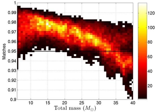
FIG. 5: Distribution of the efficiency versus the total mass. The simulation consisted of  $N_s = 40,000$  injections. The lower cut-off frequency for the injections and the BCV templates was set to 70 Hz, as in S3 BBH search.
