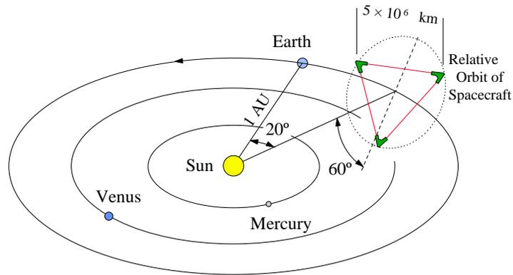
**FIGURE 3.** Schematic diagram of LISA and its orbit around the sun
