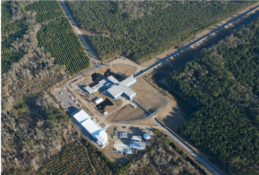
Figure 1.3: Aerial photo of the LIGO Livingston Observatory, containing the L1 detector. The main building in the center of the photo contains the beamsplitter; the two 4 km arms reach out to the right of the photo. Photo by Greg Grabeel and the author.
