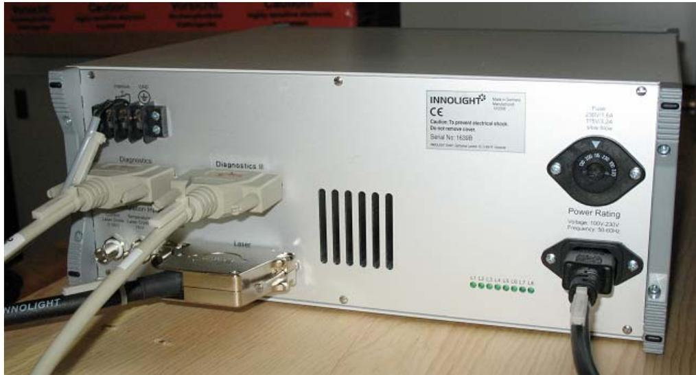
Figure 5-3: NPRO power supply back panel wiring
