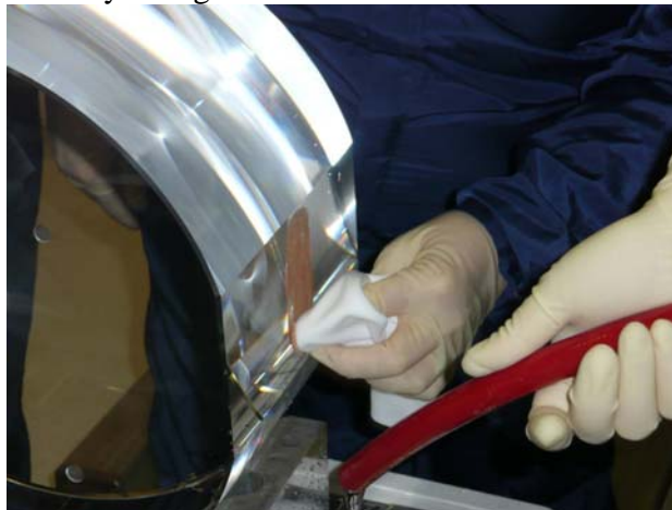
Figure 12 Cleaning the side of the penultimate mass with cerium oxide 12/12/07
