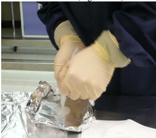
a) Dispensing the VacSeal in an aluminium boat
