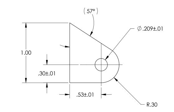
THIS PIECE IS PART OF A WELDMENT. DIMENSIONS SHOWN ARE APPROXIMATE; WELD INDUCED SHRINKAGE OR FILL, AND POST WELD ANNEALING AND MACHINING CONSIDERATIONS ARE NOT INCLUDED. SEE NEXT ASSEMBLY FOR REQUIRED DIMENSIONS FOR STRUCTURE AFTER WELDING.
