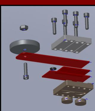
A TMD was designed and tuned to have a resonance of 153 Hz and a Q of about 6. A Viton oring, placed in slight shear, creates the loss. TMDs were then installed at the location of largest motion on the HAM-ISI blade springs.
