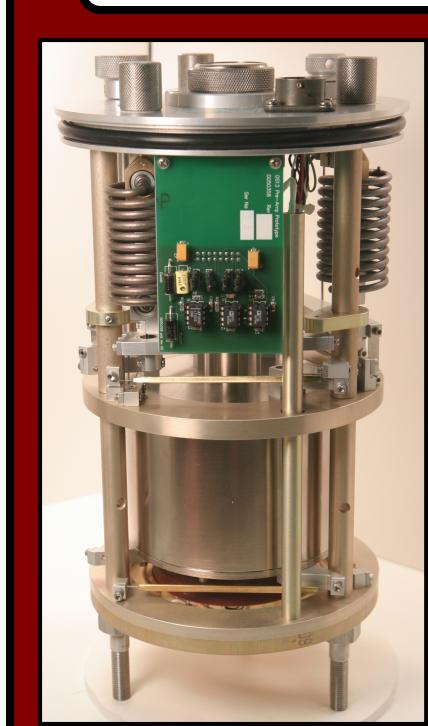
**Every LIGO HAM-ISI, seismic** isolation system, utilizes 6 **Geotech GS-13 seismometers** as sensors. A resonance in the GS-13 around 103 Hz causes a large spike in the system transfer function.
