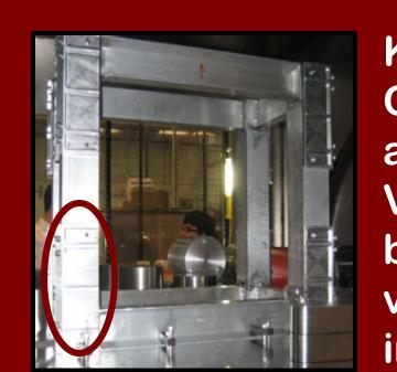
**Kurt and Calum at** CalTech also researched an alternative to struts -Viton backed corner brackets. This also is a viable option. With improved performance.
