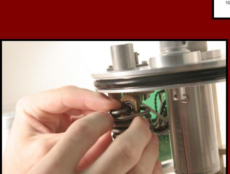
Viton o-rings were installed on all offload springs on the Stanford ETF platform's GS-13s. The o-ring was placed between adjacent coils near the fixed end.
