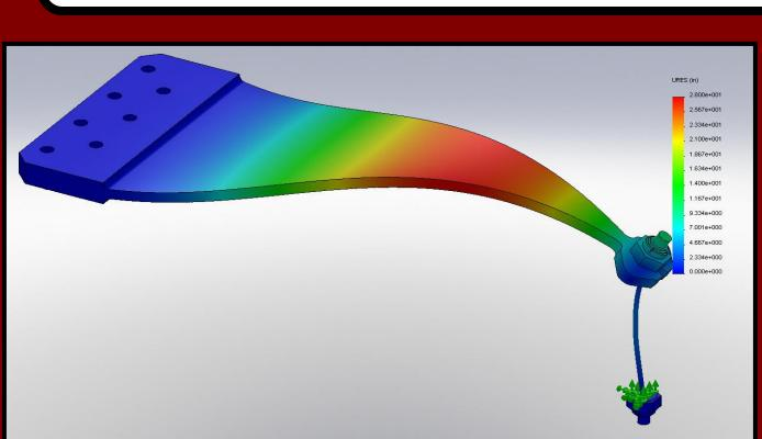
The HAM-ISI blade springs were observed to have a 153 Hz resonance mode. This was verified with FEA.
