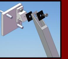
A strut was then designed which places a small pad of Viton in shear near the tip. The shear strain results were also predicted with FEA.
