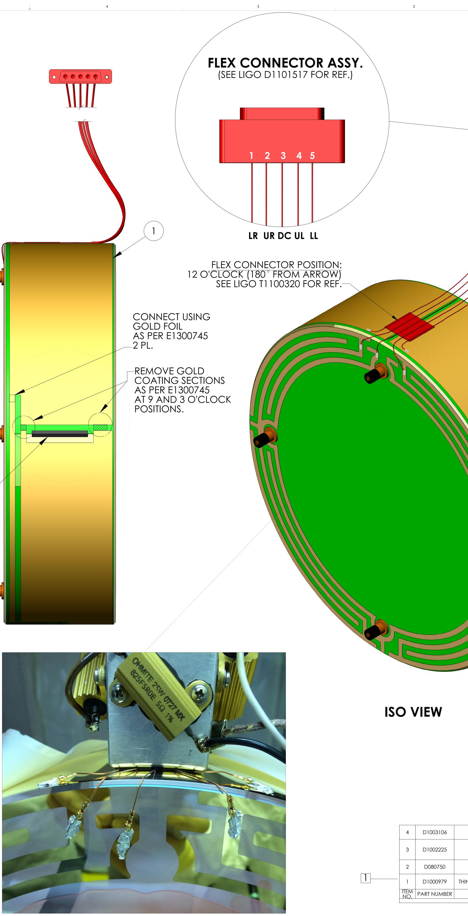
**CPY CONNECTOR TO BARREL CONNECTIONS** (REFER TO T1100320 FOR SOLDERING DETAILS)
