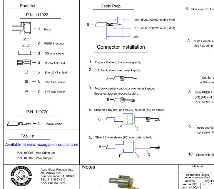
6. Slide short CKT shield (#5) onto wire, back to the SS wire sleeve (#3).
