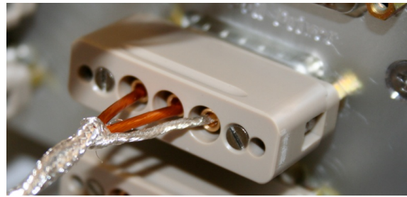
Figure – Actuator cable plugged on the feedthrough
