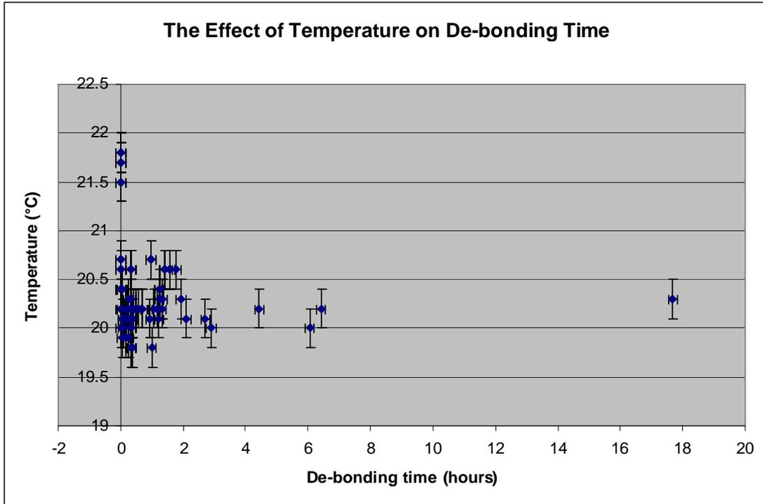
*Fig3.7. The effect of temperature on de-bonding time. As can be seen the temperature range was only 2°C and hence it is not clear that there is a relationship between temperature during bonding and the time it takes to de-bond later; although this is likely to be the case.*
