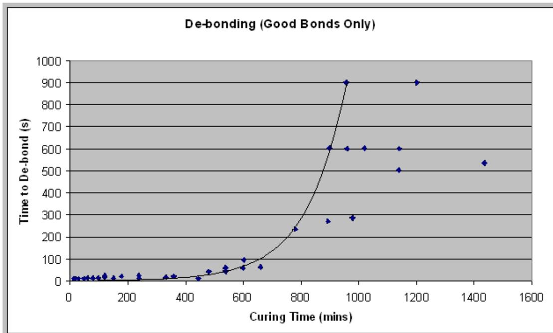
Fig 3.5 The effect of curing time on de-bonding time for samples cured for up to twenty-four hours.
