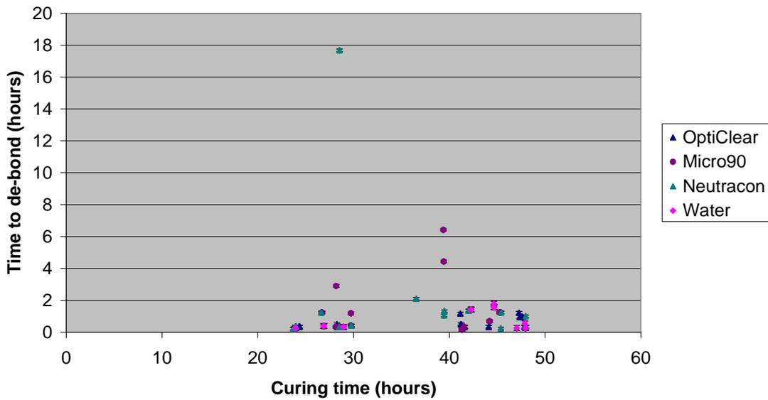
Fig3.7. A comparison in de-bonding time for OptiClear, Micro90 and Neutracon.
