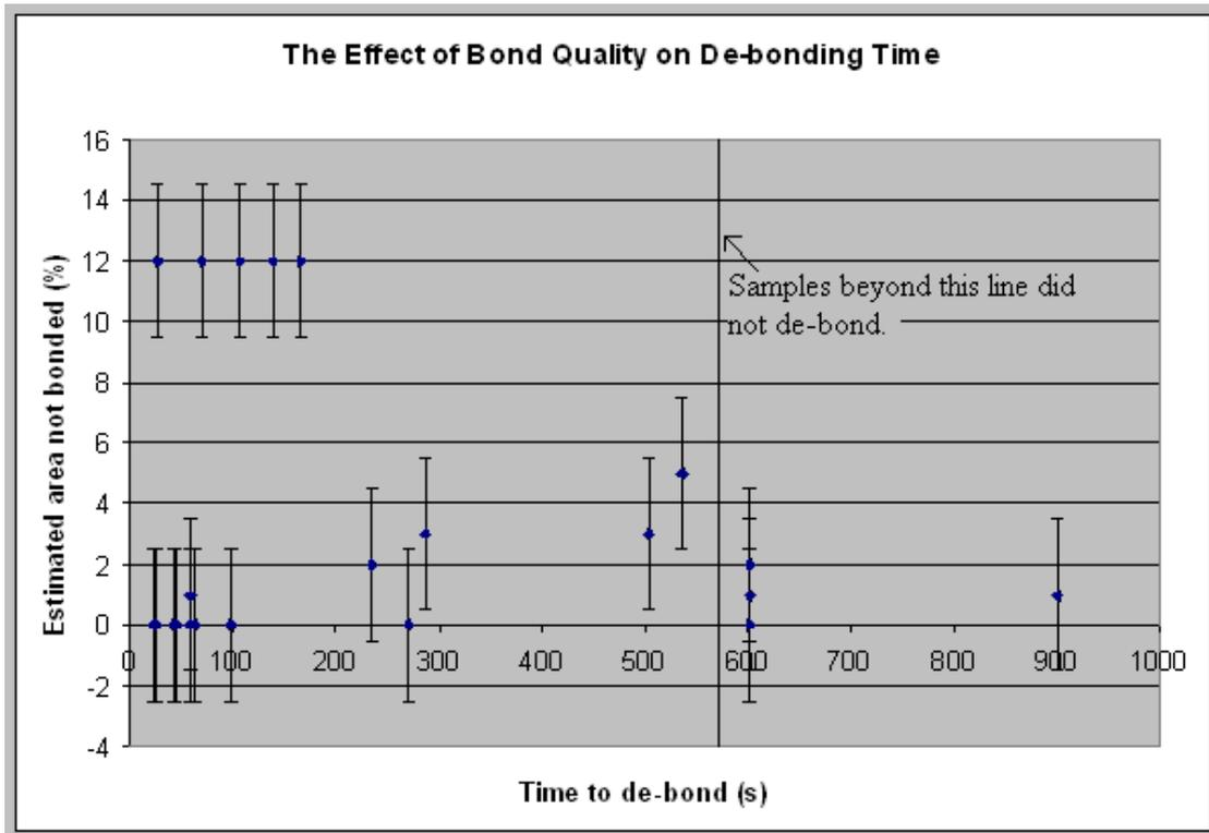
Fig 3.2 The effect on bond quality on de-bonding time for bonds aged up to twenty-four hours. Note time displayed in seconds.
