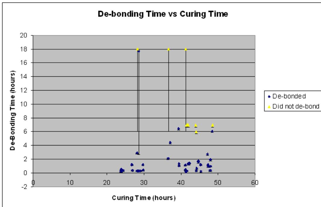
Fig 3.6. Showing the effect of curing time on the length of time required to de-bond samples.
