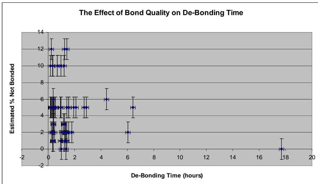
Fig3.3. The effect of bond quality on de-bonding time for bonds aged between twenty-four and forty-eight hours. Note time displaced in hours.
