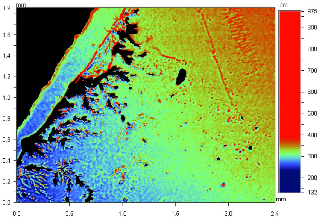
Fig3.12 Fern patterns at the edge of a disc's surface (x2 magnification).
