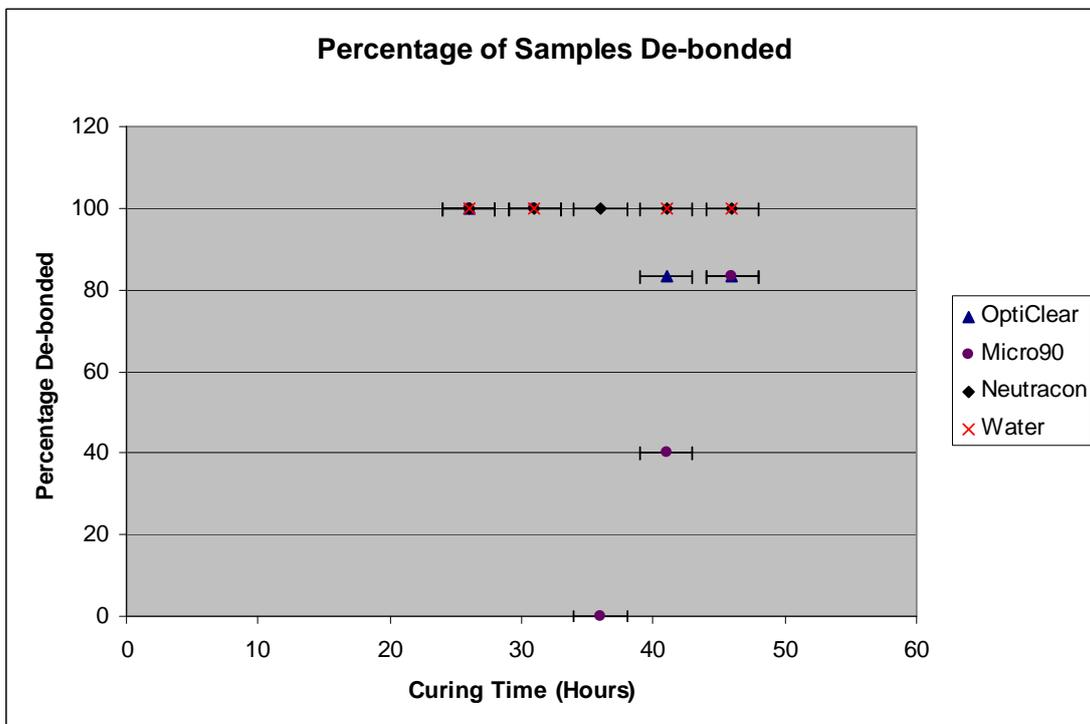
Fig3.8. A comparison of the success rates in de-bonding samples for OptiClear, Micro90, Neutracon and water.
