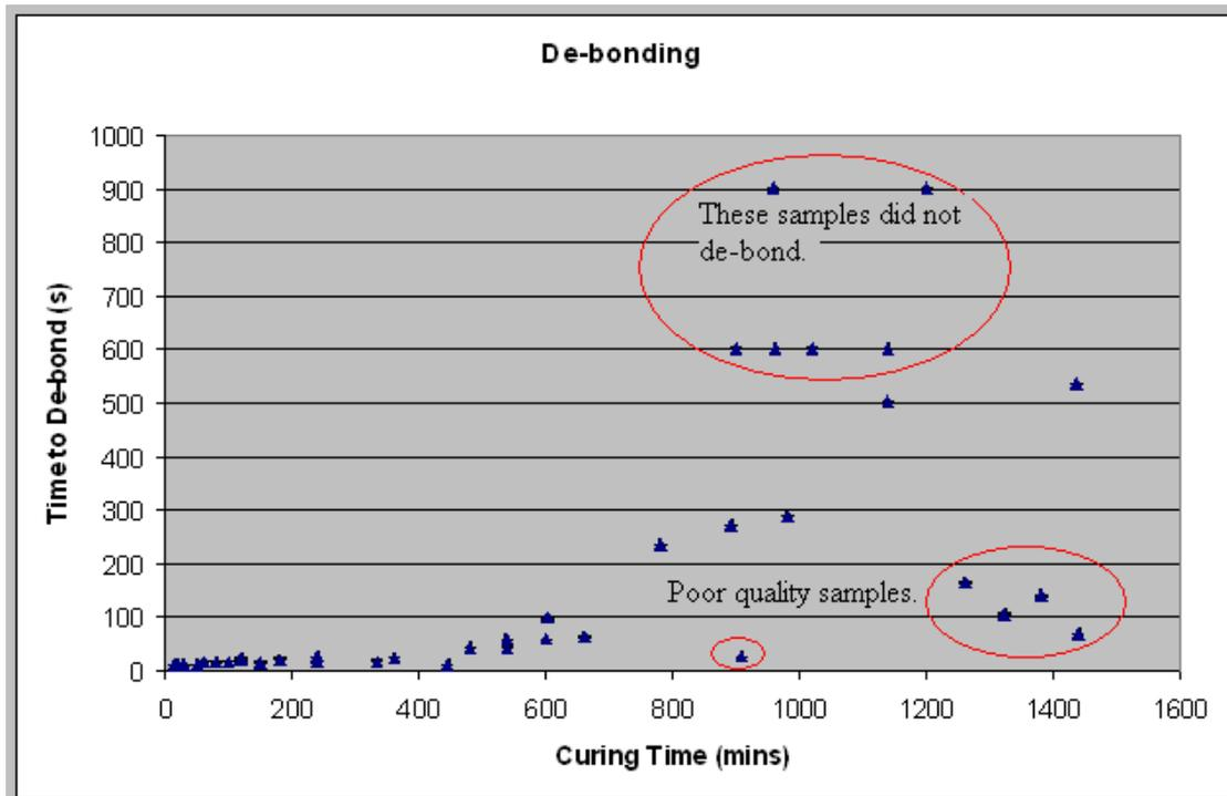
Fig 3.4. The effect of curing time on de-bonding time for samples cured for up to twenty-four hours. The samples that did not de-bond were rinsed for up to fifteen minutes. Samples are considered “poor quality” if more than ten percent of the bonding surface is not bonded.
