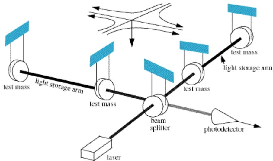
Fig1.1. Diagram of the Advanced LIGO interferometer.
