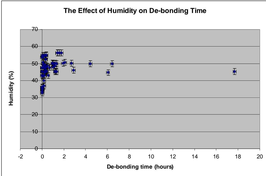
Fig3.6. The effect of humidity on de-bonding time. In this humidity range there appears not to be any relationship between the two values.
