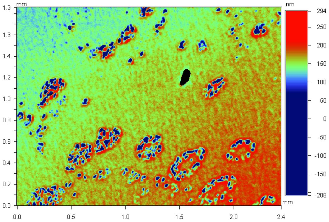
Fig3.11 Blotch patterns on the surface of a disc (x2 magnification).
