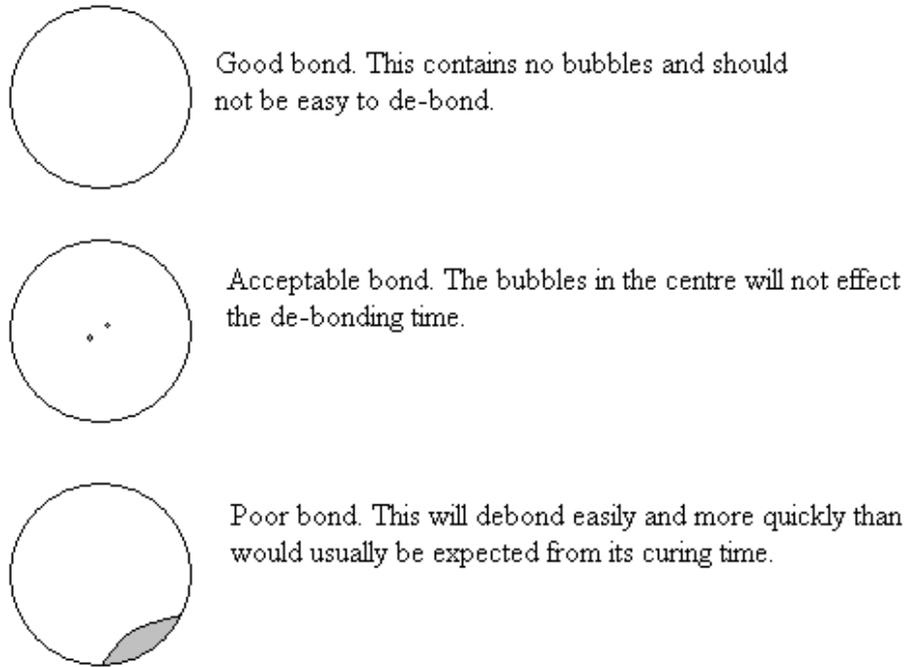
*Fig3.1. Possible bonding results and how the de-bonding time will be effected. Bubbles present in the bond do not seem to have much of an effect unless they are very large, or at the edge of the disc.*
