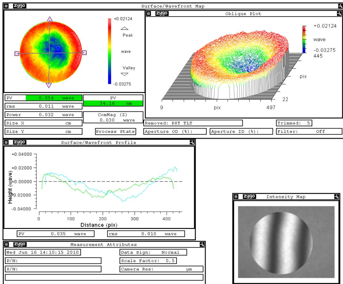
Fig 2.1. An example of the flatness data produced by Zygo interferometer. Flatness is shown in waves and nanometres by default – but can be altered so that all values are shown in nanometres (or other units as desired).
