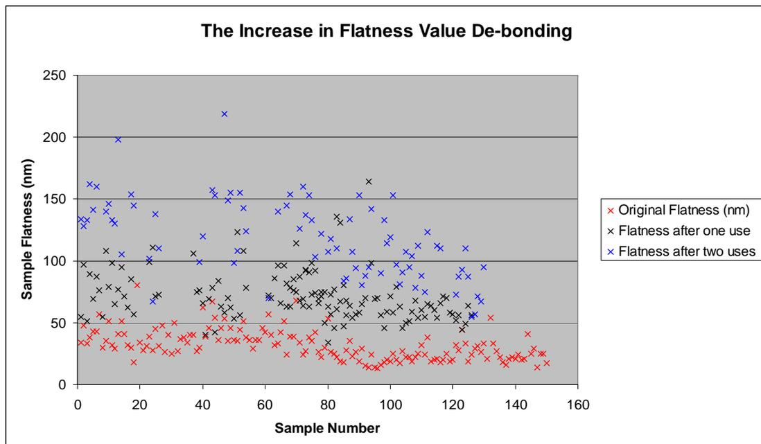
Fig3.9. The effect bonding and de-bonding samples has on their flatnesses. It can be seen that after each trial the flatness value increases.
