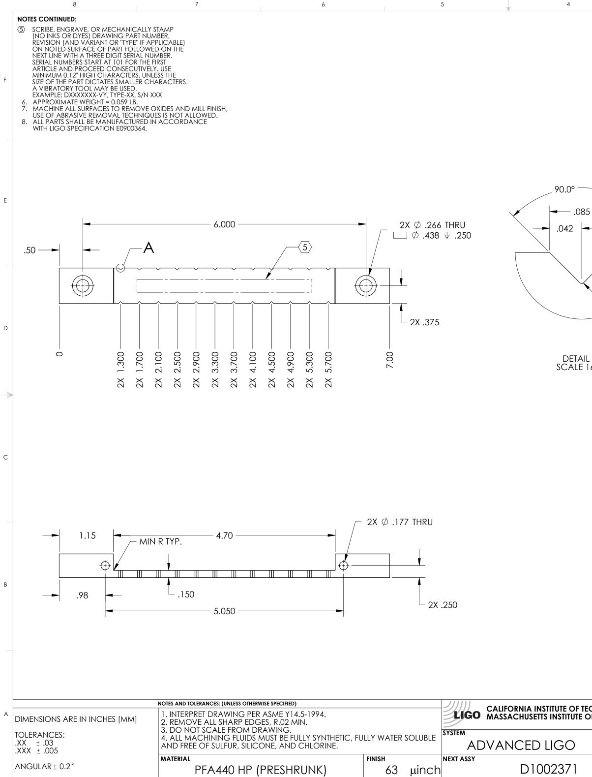
D1002372\_aLIGO\_SUS\_HSTS\_MAGNET GLUING HOLDER, PART PDM REV: X-003, DRAWING PDM REV: X-001
