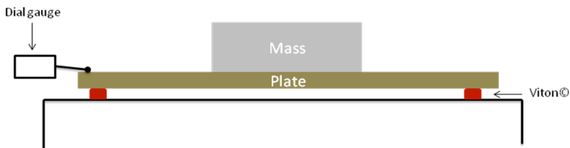
Figure 16 : General scheme of the experience used to determine the static Young modulus of the Viton®
