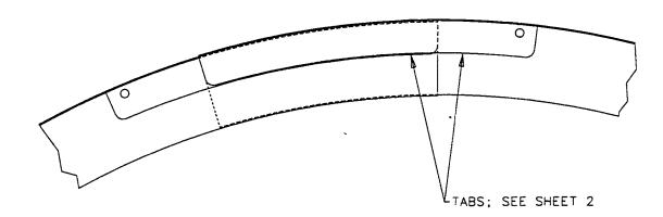
DETAIL B DRAWN INSTALLED IN MAXIMUM DIAMETER OF BEAM TUBE ( $\phi$ 49.18) 7.5 OVERLAP AT BAND
