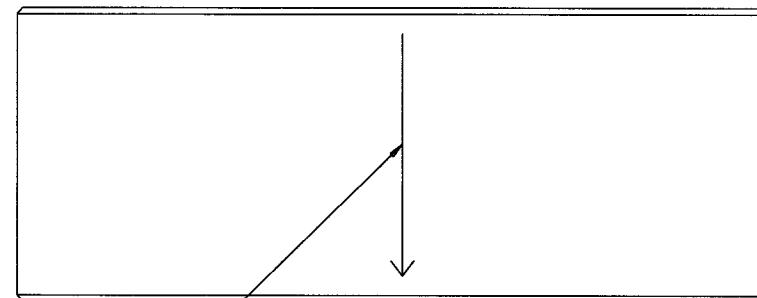
MARK "TOP" OF OPTIC (CORRESPONDING TO "TOP" ON PHASE MAPS) WITH INDELIBLE INK LINE 80 mm LONG PERPENDICULAR TO -A- WITHIN 1 mm, ARROW POINTS TO SIDE 1
