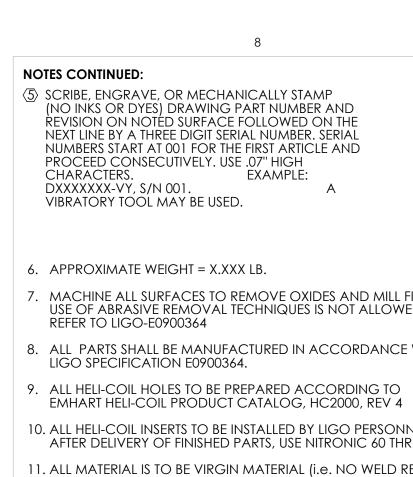
7. MACHINE ALL SURFACES TO REMOVE OXIDES AND MILL FINISH, USE OF ABRASIVE REMOVAL TECHNIQUES IS NOT ALLOWED.
