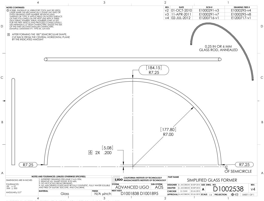
D1002538 SIMPLIFIED GLASS FORMER, PART PDM REV: X-003, DRAWING PDM REV: X-005
