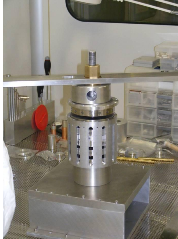
Faraday magnetic system during the assembling
