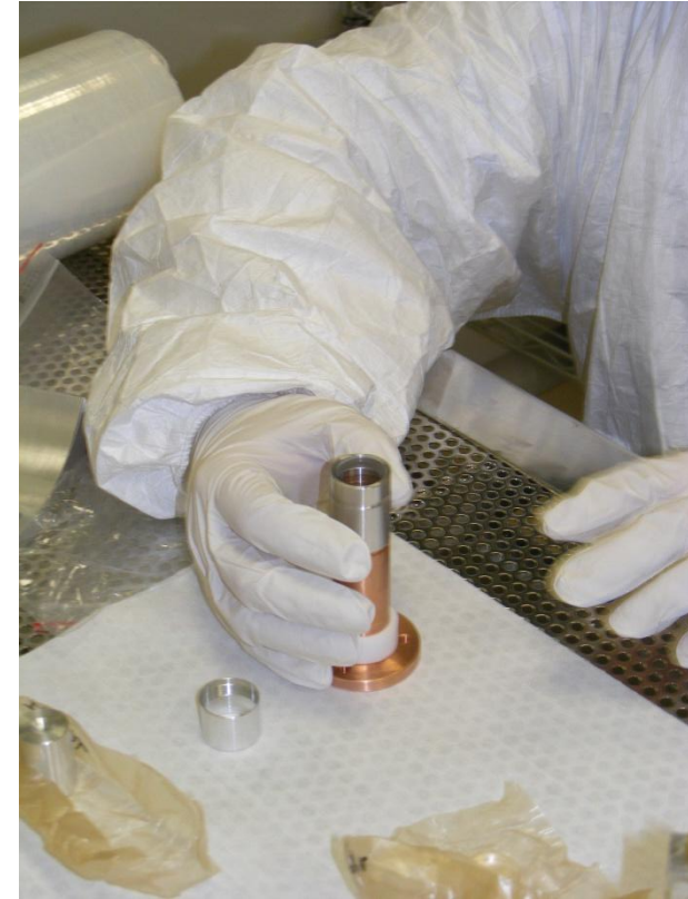
TGG crystal installation in its copper holder
