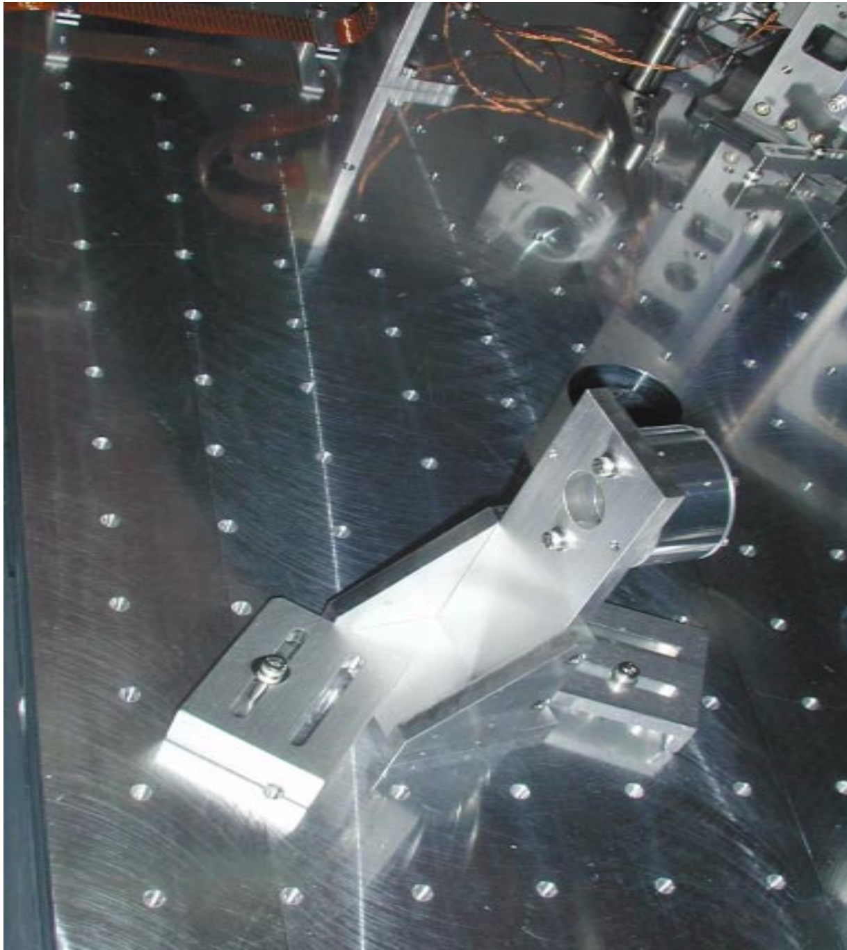
HAM7 MC3 Optical Lever steering mirror on West side of table. North is at the top.
