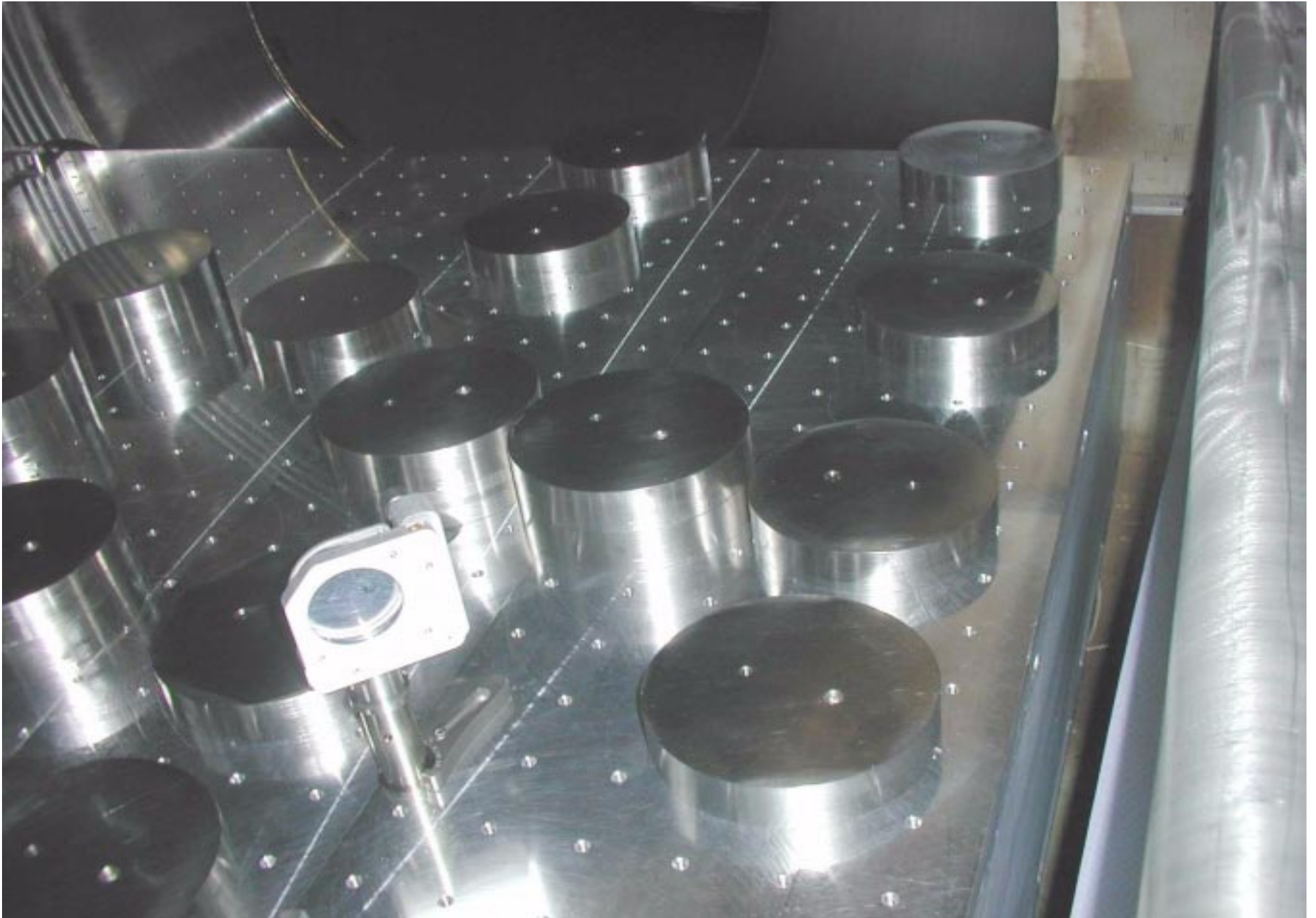
HAM7 SW corner with counterweights and MC Reflected Beam steering mirror.
