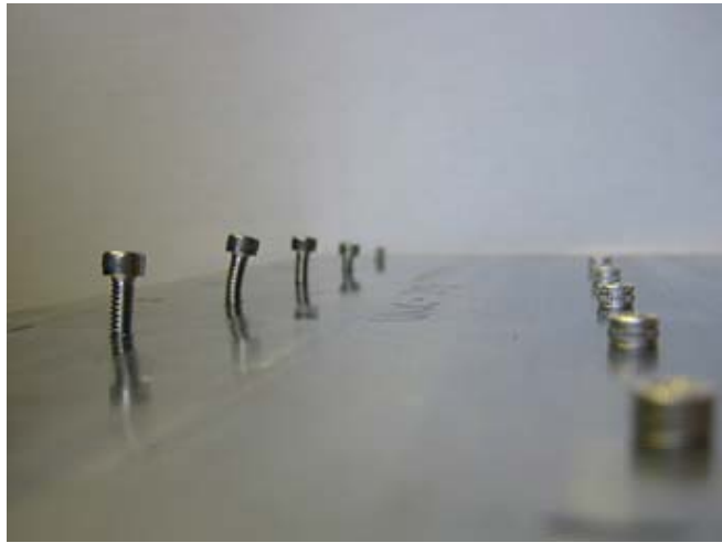
Figure 2.24 Screws deformed after freezing
