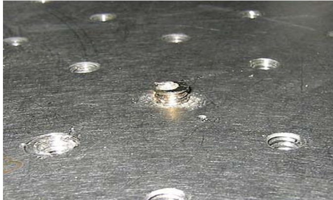
Figure 2.21 Frozen steel screw in a stainless steel optical table
