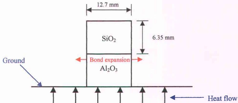
The heat source is placed under the ground so that the flow goes towards the sapphire first and then through the fused silica. Since the model is symmetric, we can expect an expansion of both parts such as the one drawn above in red.
