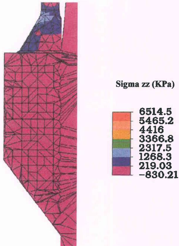
As the previous one, we are now very close to pure shear in the bond because of the geometry of the ear. The maximum normal stress is very close to zero.
