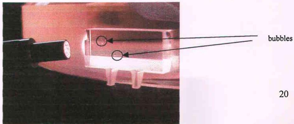
The few bubbles observed after the bonding could be dangerous as they represent stress focus points.
