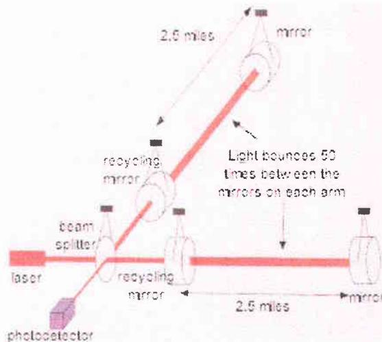
The "Fabry-Perot" mirrors (recycling mirrors on the drawing) are considered here as test masses. Since wires suspend them, one can assume that they also are free masses from a mechanical point of view.
