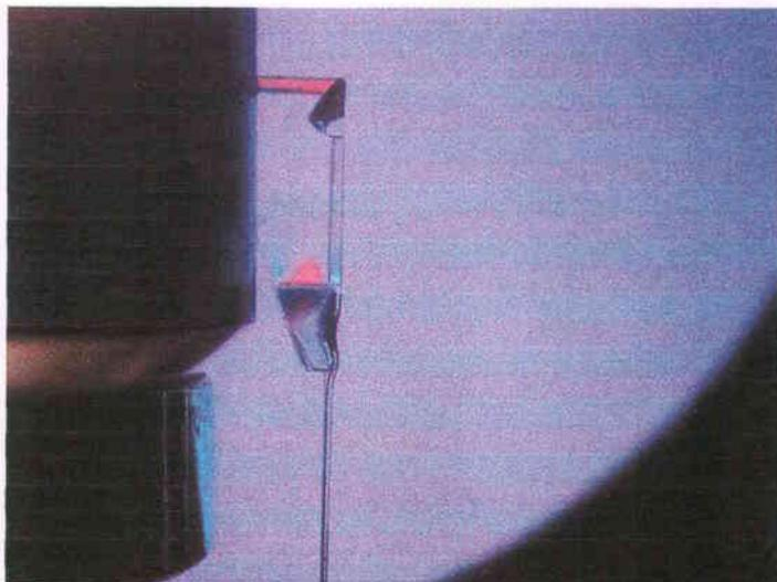
We can already see several color spots where we expected stresses focuses when loading the fibers a little more. Most of these spots are due to the geometry of the bond, especially at different edges and corners of the ear because of geometry angles.
