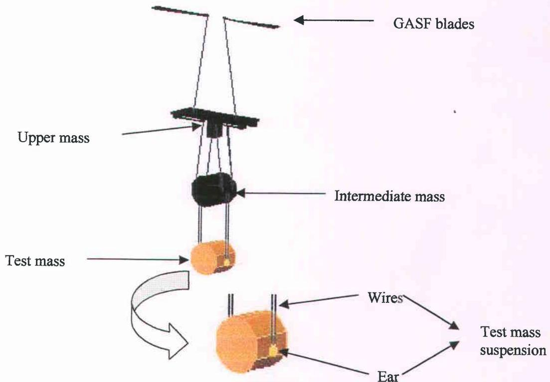
As one can see, on both sides, the test mass is suspended to the intermediate mass by two wires welded to an “ear” which is itself bonded to the mirror. The three
