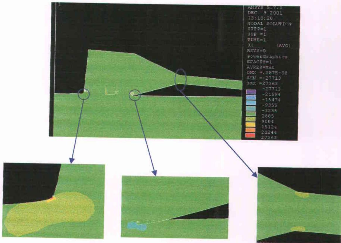
The  $\sigma_{xx}$  distribution (x along the bond) is uniform in the suspension. Regardless to the bond, we have two sensible points at the extremities of the interface. A maximum stress is located at the left extremity (point P, cf. 2.4) and a minimum at the right extremity. The minimum has actually the same intensity that the maximum one but
