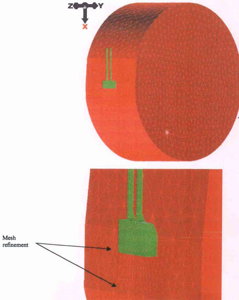
Using the FEA editor, we will perform a static analysis. The material specified is the same for all the different parts of the suspension: fused silica. The fibers are clamped on their top section and the gravity is applied at the center of gravity of the mirror. After performing the analysis, Algor gives the following shear distribution at the surface of the model:
