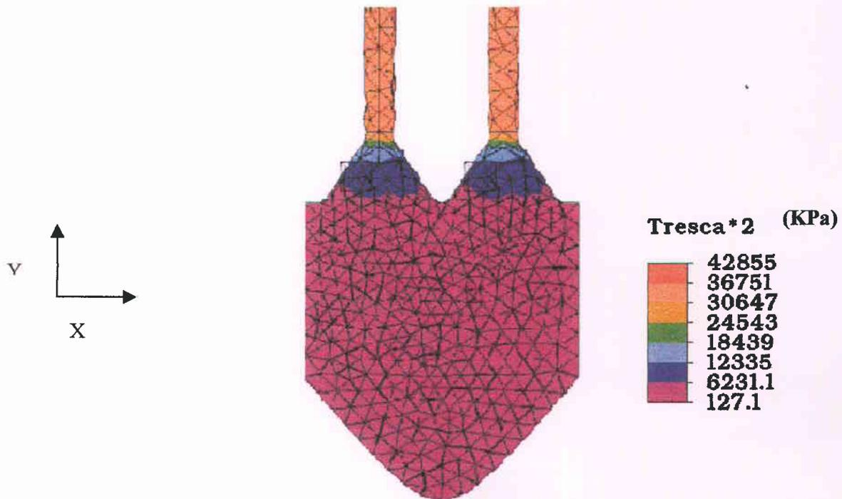
The stress distribution seems constant over the bond area. The maximum stress could be evaluated at 3.1 MPa.
