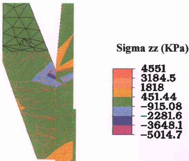
It seems like the stress applied by the mirror on the ear is larger now, especially regarding to the compression (blue colors). According to the color scale, we can estimate the maximum compression stress at  $-3.65$  MPa.
