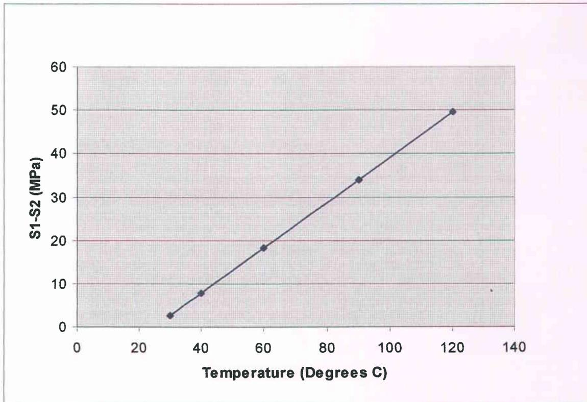
According to the viscoelastic behavior of the bond, the stress varies linearly with temperature.
