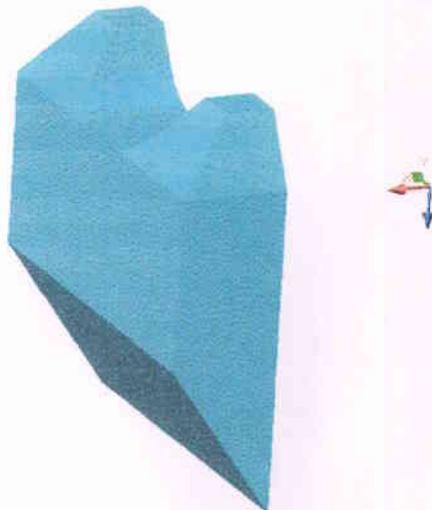
Due to the new mirror design, the bonding surface and the legs are now in the same vertical plan.
