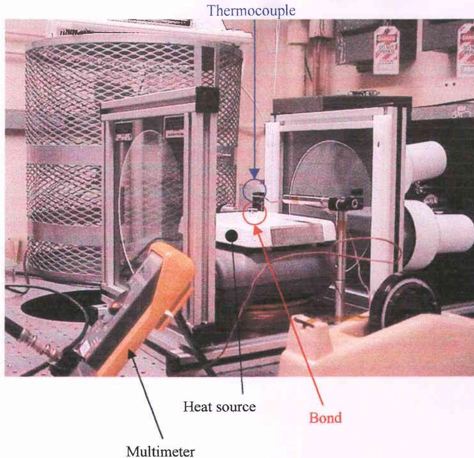
A plate generates the heat so that the flow goes through the sample from the bottom. This plate can heat the sample up, cool it down or maintain it at a constant temperature. The thermocouple is in contact with the top of the sample, its voltage varies with temperature. This voltage is transmitted to a multimeter, which will convert it into a temperature in degrees Celsius.
