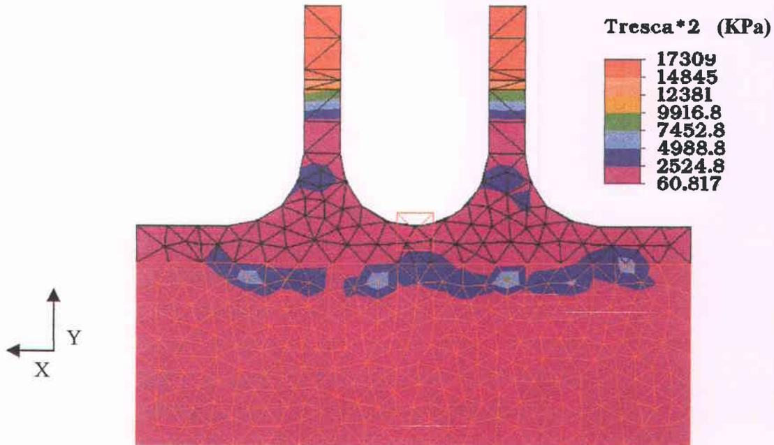
The shear distribution varies from the bottom to the top of the bond and it is vertically symmetric. Here again, the maximum shear stress (about 3.7 MPa) in the bond is very low compared to the breaking stress of this layer. We can note some stress focus points (in bright blue) at the upper limit of the bond area, which is the most sensitive part to the shear in the bond. The maximum stress is situated at the welded part of the legs.  $\sigma_{yy}$  is displayed on figure 5 given in annex.
