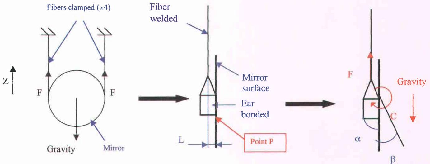
Assuming that the main efforts in the suspension are vertical along the x-axis, we can expect shear stress as the most important stress in the bond.
