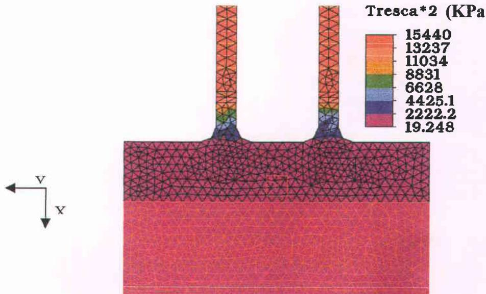
The shear distribution is constant in the bond. We can observe a variation of the stress along the fiber, especially after the welded part, the stress reaches its maximum value (7.72 MPa). The value of the shear in the bond is varying between 0.1 and 1.11 MPa, which are very small compared to the breaking stress of the bond (20 MPa).
