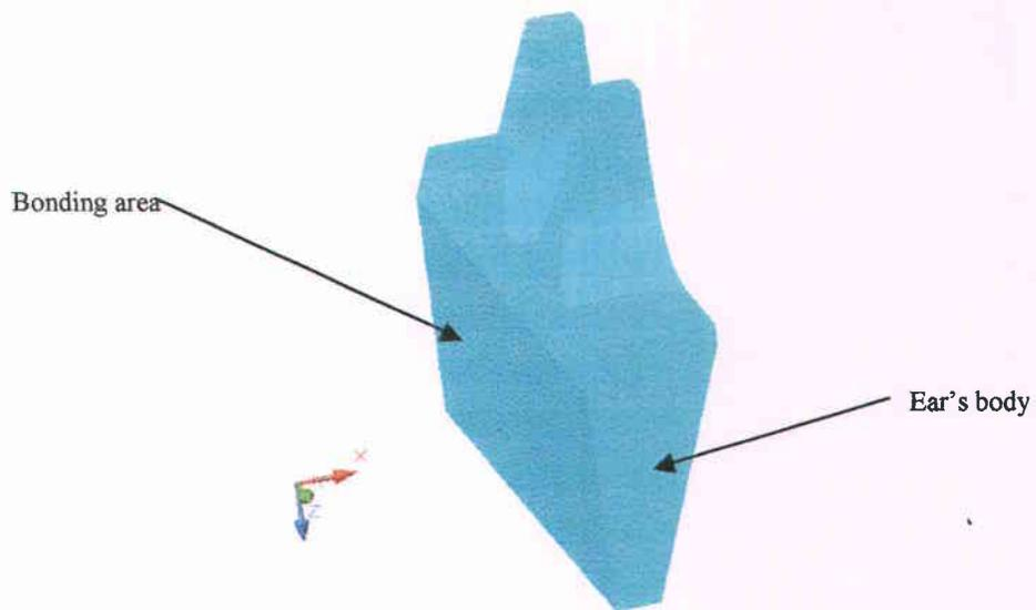
The main difference with the previous design is the trapezoidal shape of the ear's body instead of a prism shape.
