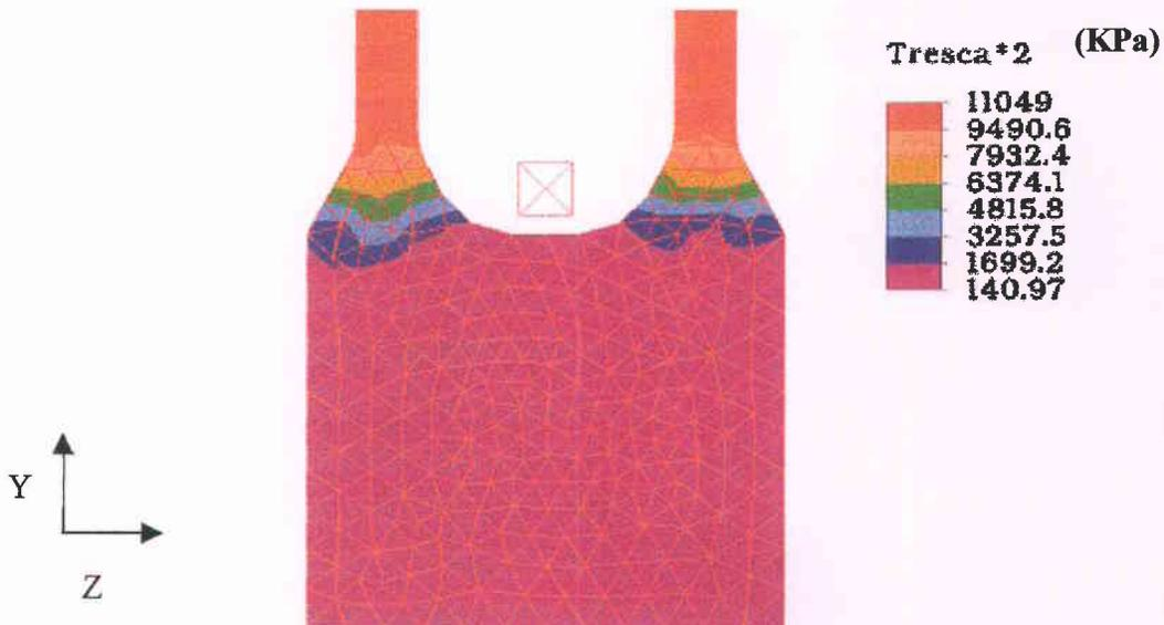
The shear in the bond looks constant. The distribution is similar to the first bond model one. The maximum shear stress is about 0.85 MPa.
