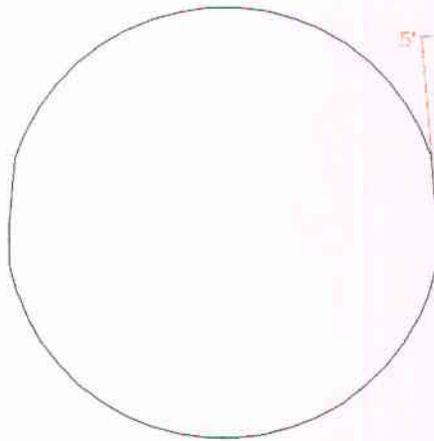
5° will be enough to avoid the contact between the ear and the mirror side but at this time, we don't know if it will be also enough to weld the fibers without damaging the mirror. Burning the mirror while welding the fibers could decrease its quality factor. Machining a larger angle won't be a problem anyway. The important thing is to keep the idea of building this inclined plane on the mirror's sides.
