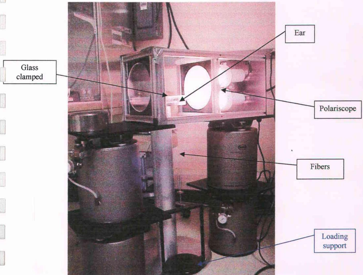
The loading support was machined especially for these experiments; the system is directly glued on the fibers:
