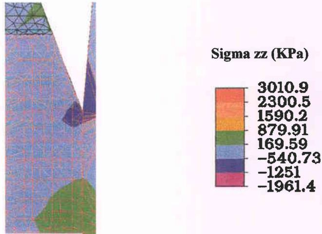
By referring to the color scale, we can easily see the effect of the mirror on the bond, pushing on the top and pulling at the bottom. The maximum compression stress applied by the mirror would be  $-1.25$  MPa according to the color scale. This is what we have to minimize.  $\sigma_{xx}$  is displayed on figure 3 given in annex.
