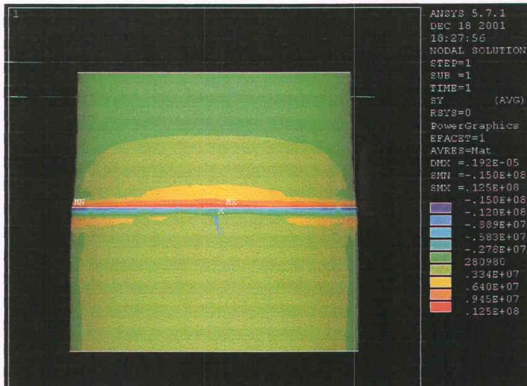
As we expected, the maximum stress is situated at the interface. The deformed shape reveals that the sapphire is applying stress to the fused silica; we can notice that the sapphire guides the deformations of the fused silica.
