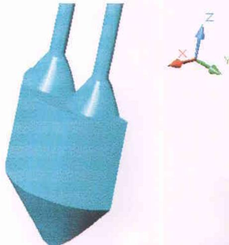
This model is composed of three cones and one cylinder, and the fibers have a circular section (2mm of diameter). The mirror is machined the same that the third model one.
