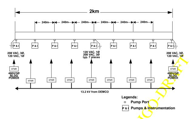
DC power supply layout (top); AC power distribution for heater jackets, pumps and instrumentation (bottom)
