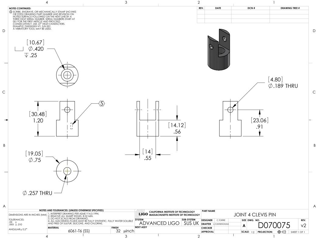
D070075\_ALIGOSUS\_UK\_PROOFBOUNCETESTERFORFIBRE\_JOINT\_FOR\_CLEVISPIN, PART PDM REV: 00, DRAWING PDM REV: 00
