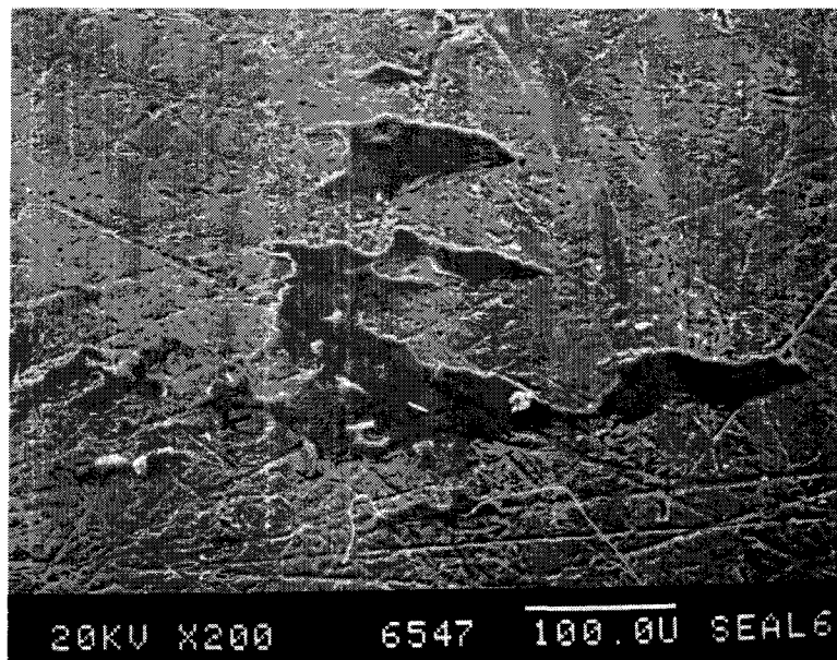
Figure 2. 200X SEM Image of Aluminum Dumbbell Bonding Surface
