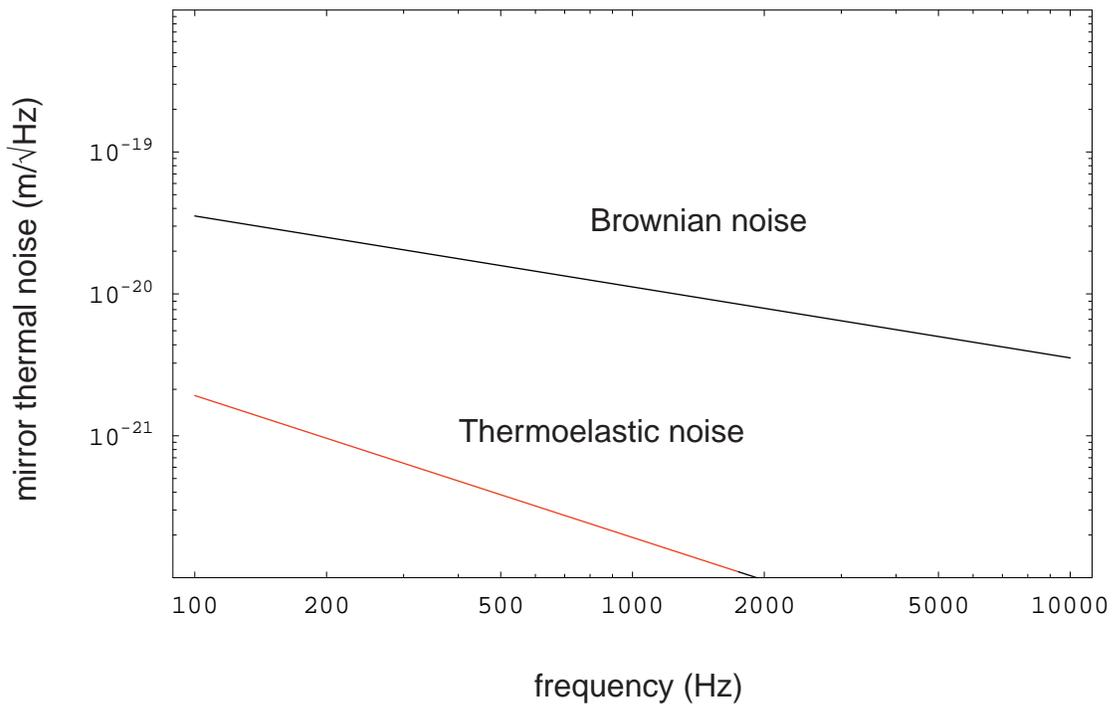
Figure 3: Expected noise in the proposed 40-meter with fused silica mirrors. This should closely mimic LIGO's thermal noise curve. Note that this scale is the same as that of Figure 4.
