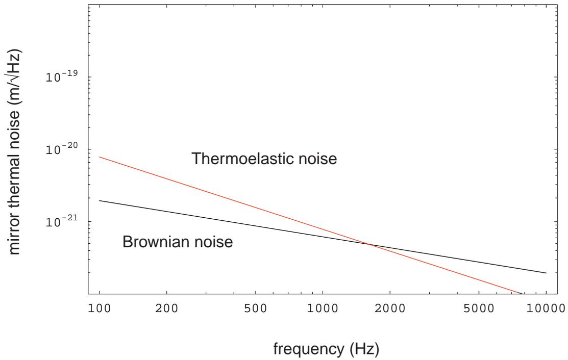
Figure 4: Expected noise in LIGO with sapphire mirrors and unchanged spot size. Thermoelastic noise is not nearly so much of a problem as in Braginsky's plots, because he underestimated our spot size.
