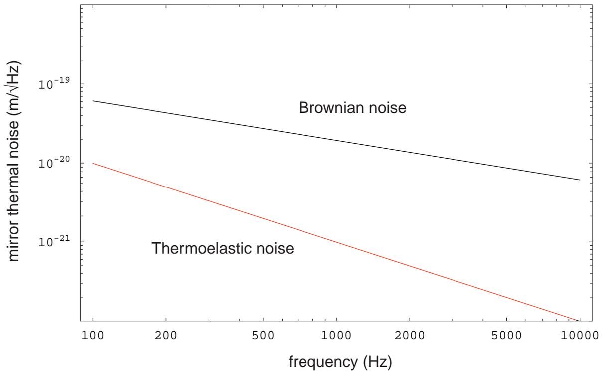
Figure 7: Could the old 40-meter have seen thermoelastic noise? Not likely, if its g-factor were 1/3 as is LIGO's. Brownian noise would still have been dominant.
