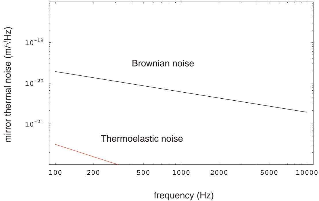
Figure 1: Expected noise in LIGO with fused silica mirrors. Brownian motion dominates.
