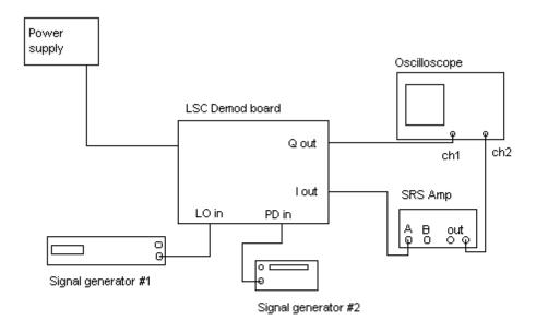
Power supplies provide  $\pm$  24 V, and +15V either to P1, or to the test points. Typical currents are 180 mA on the +15 V line, and 30 mA on each 24 V line.
