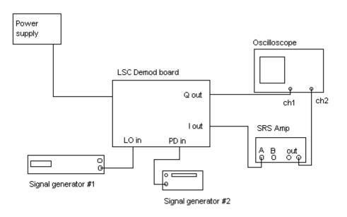
Power supplies provide  $\pm 24$  V, and +15V either to P1, or to the test points. Typical currents are 180 mA on the +15 V line, and 30 mA on each 24 V line.
