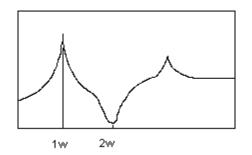
A resonance should be present at the operating frequency of the diode  $(1\omega)$ , and a notch should be present at twice the operating frequency  $(2\omega)$ . The second resonance is not required, and is a secondary characteristic of the circuit.
