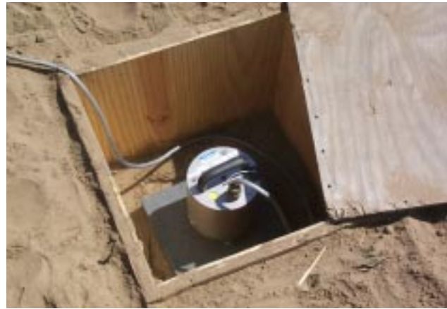
Figure 1. Seismometer in pit at site 2.
