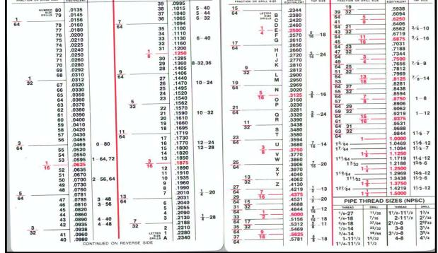
picture, left); Catalogue item number 1317. Note that all above decimal hole diameters have corresponding fractions or drill sizes.
