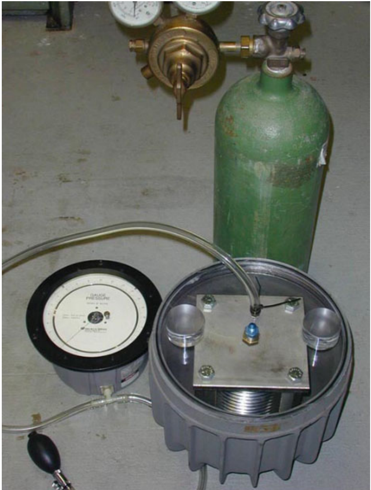
T030124-00-D Hydrostatic testing results of bellows for the HEPI actuator Page 5 of 7
