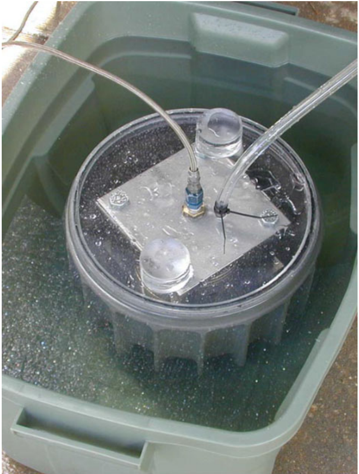
T030124-00-D Hydrostatic testing results of bellows for the HEPI actuator Page 6 of 7
