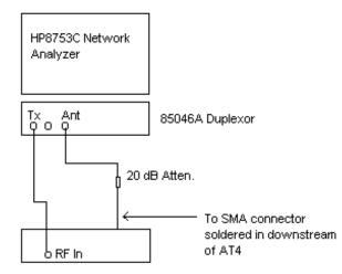
This test is performed with the HP8753C or HP4195A Network analyzer. A signal generated by the network analyzer is input to the AM stabilizer at the RF Input jack, J3. The return signal is taken from an SMA connector (with a short section of semi rigid coax) soldered into the circuit downstream of AT4.
