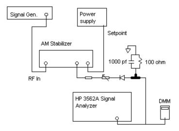
The output signal is taken from the RF OUT TO EOM jack, run through a fixed attenuator ( if required), a variable attenuator, and an ACSP diode detector. The filter after the diode is placed in the circuit using a BNC "T" connector. The diode voltage is read on the DMM.
