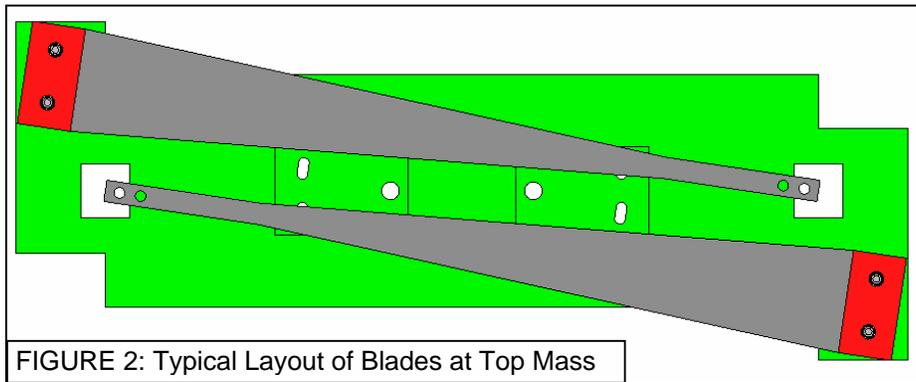
FIGURE 2: Typical Layout of Blades at Top Mass
