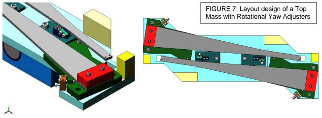
• The **OSEM coils** must be adjustable in x, y and z directions, and have adjustment for pitch and yaw.
