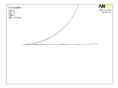
The second result looks much flatter. Note that the tip is turned up – this is as expected because the region near the tip is not part of the triangle. Therefore it does not have a constant bending radius (or stress). This is clearer in a stress plot:
