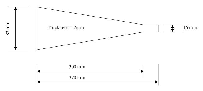
For a stress of 600 MPa at the root, the load is
