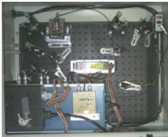
Figure 4: A photograph of the photon calibrator enclosure.
