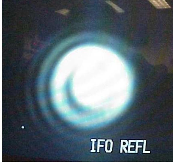
FIG. 4: The effect of mode mismatch into the cold recycling cavity. Image taken from a CCD camera at the reflected port.
